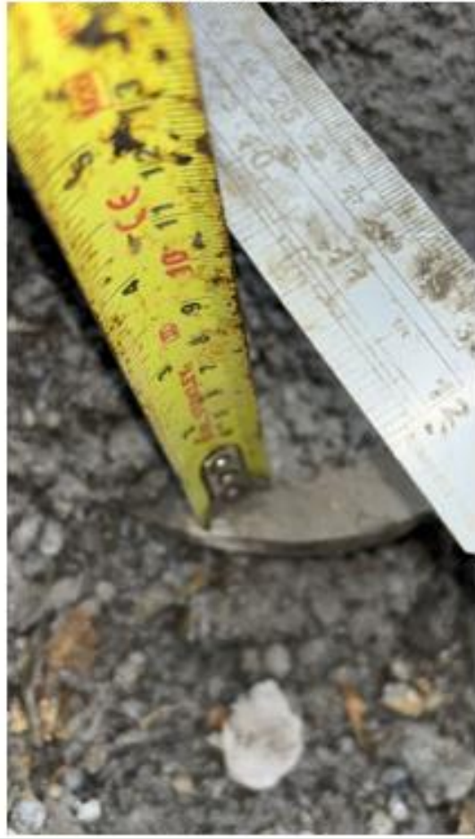
Cover 109mm Transverse square rebar
