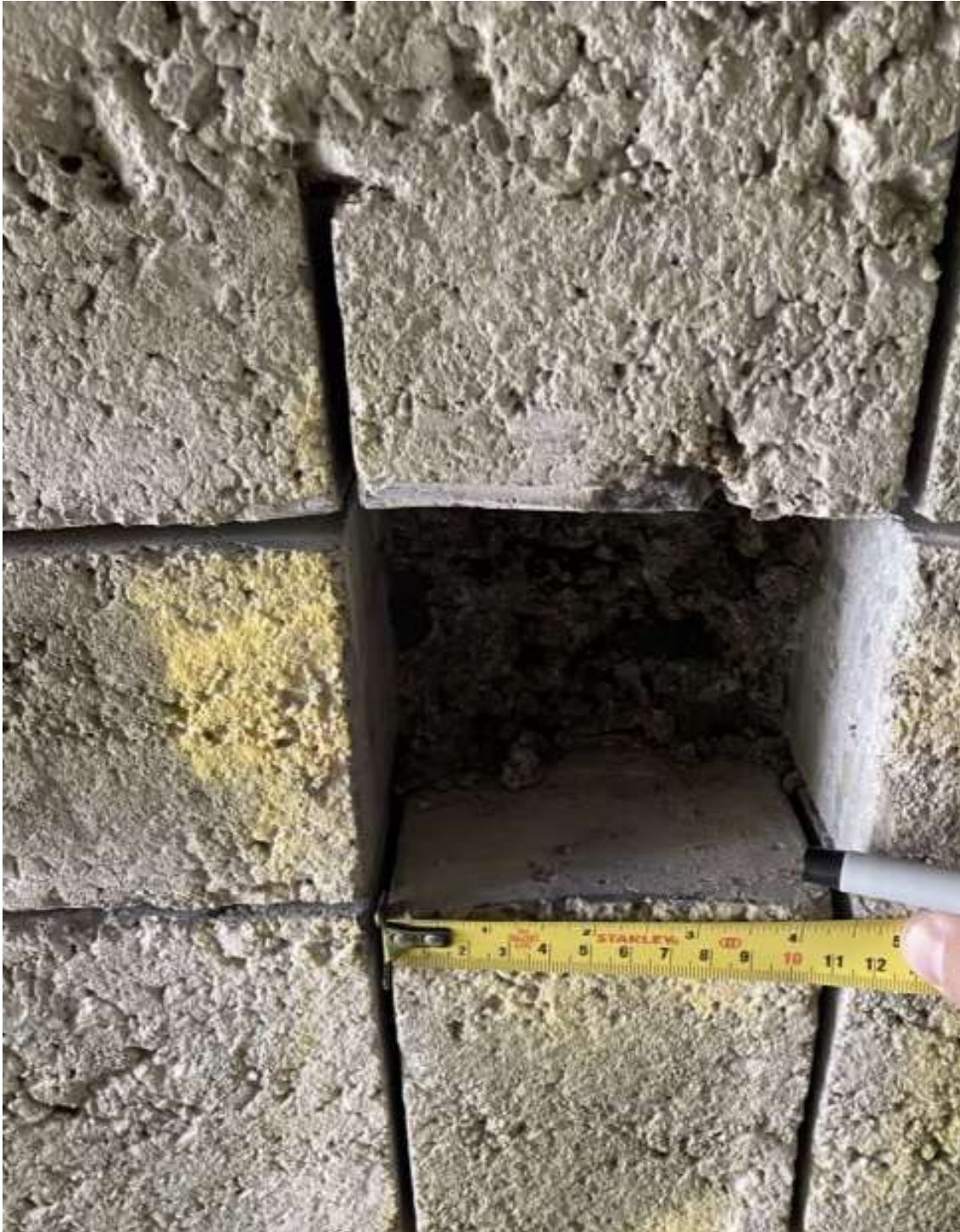
Figure 48: Carbonation sample consisted of 100mm x 100mm x 80mm cuboid
