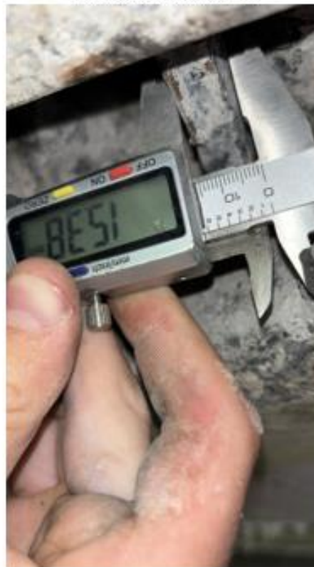
Transverse rebar 15.38mm
